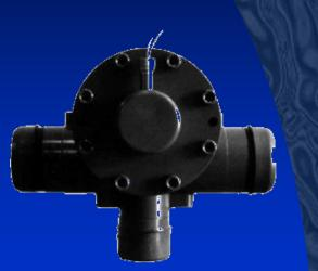
Volumetric Liquid moving through meter causes rotor to turn in proportion to flow rate Straight pipe requirements Changes in flow rate and viscosity can have large effect on accuracy Some moving parts
